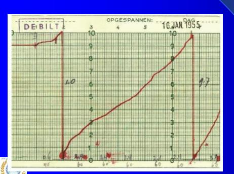
The rainwater collected by the collector is led to the float chamber. The float is having central stud on which pen assembly is fixed. The pen is moving over a daily chart wound over a clock drum. After every 10 mm of rainfall syphoning occurs and recording of rain starts afresh(IS 5225-1969)
